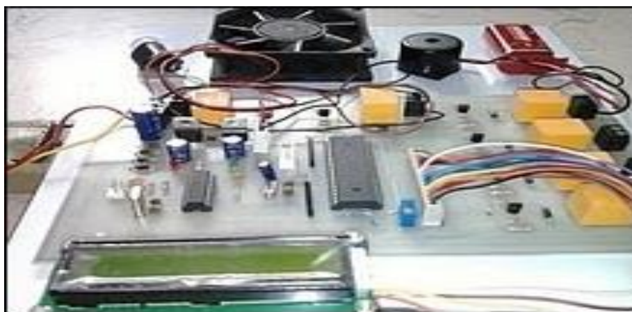
Fig.3 Real implementation of Home automation system
